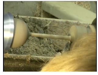
Completing the bottom and just a little sanding finished the goblet demo.
