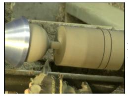
Next up was the shaping of the stem and the bottom with the R4 tool.
