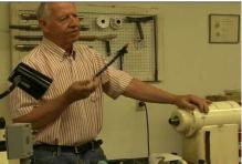
Lastly he shared about the use of a flexible air hose to cool sand paper and help remove the dust.
