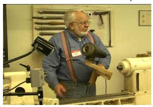
Ken put a chuck on the ONE WAY and talked about being safe when the jaw corners are exposed over the chuck body. Losing a fingernail or worst, he suggested using a couple of turns of masking tape fills the gaps so the accident is avoided. (Ed. Note: I like to use blue painters tape and have also use the red painters tape just to make is eye catching before I place my hand in harm's way.)
