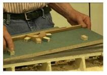
To remove the glue spray with denatured alcohol; let it set for a minute or two and apply a sideward force to dislodge the glue from the board.
