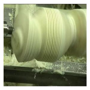
Next came the process of placing the wood on a different axis. Clay lead and in depth discussion on the balancing and placement of the center points to get the correct position for the next cuts.
