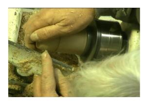
Several tricks here could help hold the top to the base – a tissue paper wedge or painters tape. John's best suggestion was to use a smaller tool and use your fingers to apply pressure to the top .The small tool allows for less metal touching the wood when you pull cut from the center to the edge. This pulling cut and the hand pressure apply enough force to hold the lid on the jam chuck.
