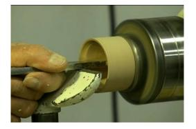
Using a parting tool the lip is formed and a sharp round nosed scraper is used to finish the coring of the top. Light cuts and a fluid motion smooth out the bowl gouge marks.
