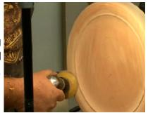
Next an application of Denatured Alcohol to show any scratches. Finding no sanding marks or other sanding needs David declared the front good and reversed jam chucked the platter to work on the bottom.
