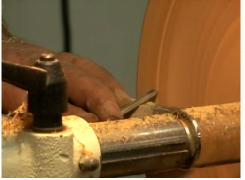
Using a 3/8" gouge, a custom made tool rest and the tailstock brought up tight for safety David started to define his rim and edge for his detail. Taking his small sharp gouge he moved slowly around the corner to have full control of the tool in riding the bevel and the cutting edge. He prepared the rim for the bead he was going to establish after he removed the bulk of the wood from the center of the platter.
