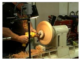
Now the most important part is the sanding. "I start at 120 grit because I know that starting at 120 grit it will come out perfect every time... I'm using a 5" hard sanding disk and keeping it tight against the platter cutting in a planeing motion. "He wants it nice and flat. From there He quickly sanded through the grits 80,150,180,220 and 420 on a medium 5" pad going in one direction for one grit and changing the direction on the drill for the next grit.
