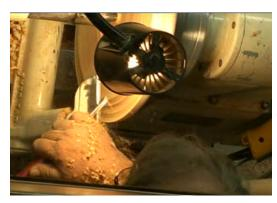
Once reset he starts at the rim and carefully works the front edge in width and appearance.
