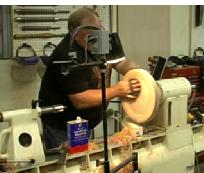
Next comes defining the foot and making the necessary controlled cuts to finish the design.
