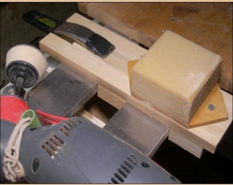
with the Maine Woodturner discount) that filled the bill! As the photo shows, a few scraps of wood and a spring clamp makes the assembly immobile on the ways of the lathe and one takes a fast swipe at the cleaner without changing one's (two handed) grip on the sander. It is a simple gear change that has made an unpleasant task go easier and quicker.
