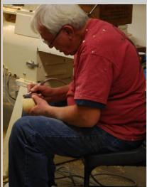
wood. The dentist drill is a 300,000 rpm cutting instrument using diamond bits just like the dentist uses. Sitting on his dentist chair John drilled holes in the
