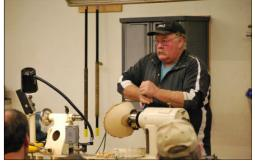
He reversed the blank and placed it in the Stronghold Chuck. Using a medium speed and slow cuts David first found the bevel of the gouge and then moved to air before twisting and slightly pushing forward to engage the cutting edge of the gouge.
