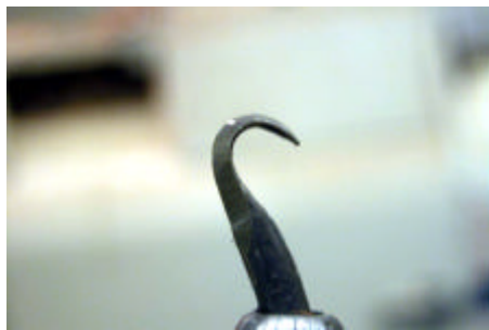
The hook tool Hosaluk uses for hollowing. (Photo by Jorge Castaneda
