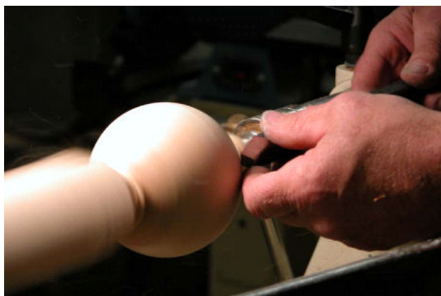
Free hand shear scraping
