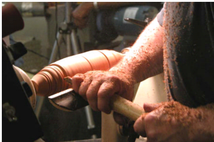
First steps of shaping Hosaluk’s signature box. (Photo by Jorge Castaneda)
