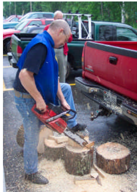
Rough shaping the bowl blank with the chainsaw.
