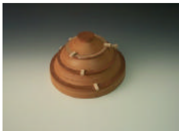
A typical glue-up using Stephen’s ring method.
