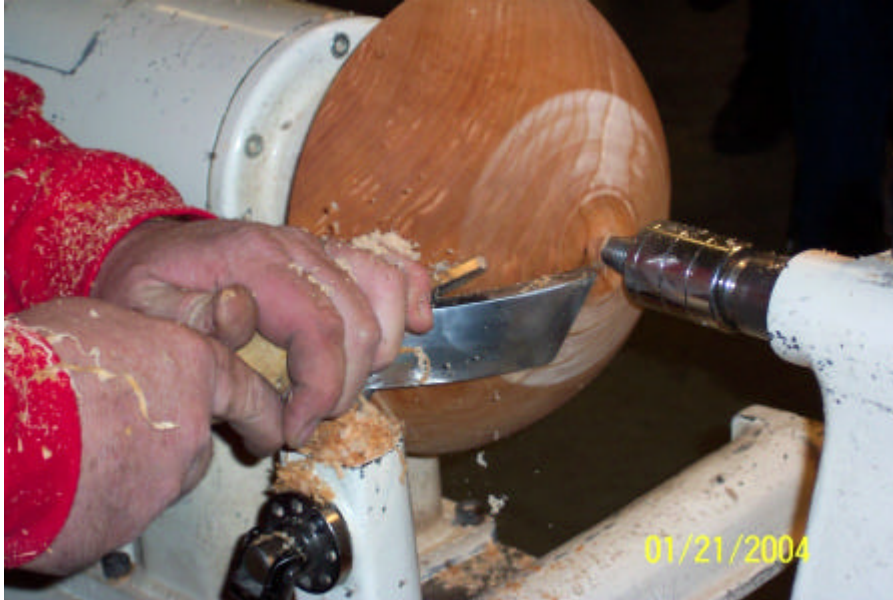
Dave both bevel cuts and scrapes to get a fine finished surface on the bowl. The better surface he gets with the tool, the less sanding he has to
