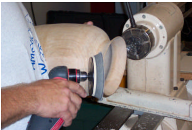
Hoover reaches under the lip of a thin cut (1/16") hollow vessel with a 5-inch mandrel and a soft pad.
