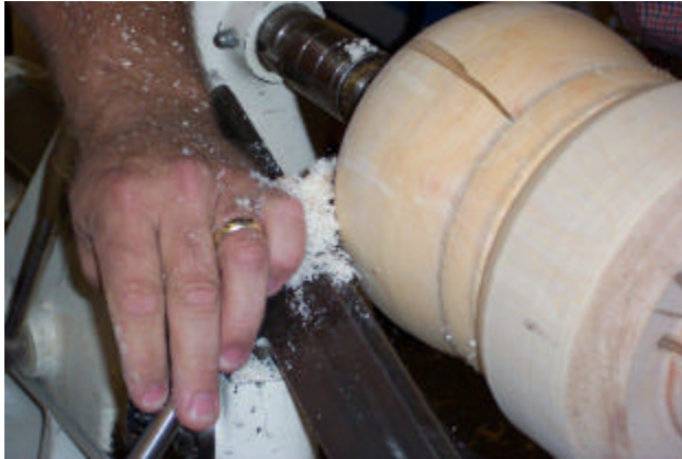
Very fine shavings come off the tool when sheer scraping is done.
