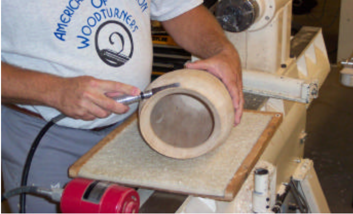
Bruce uses a detail sander to keep edges
