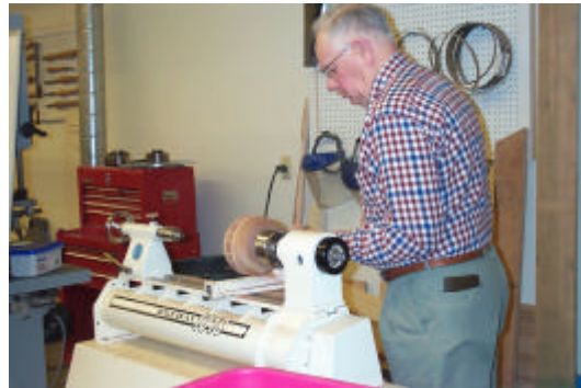
Truing up the form on the lathe.
