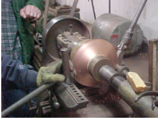
Copper being spun over form.
