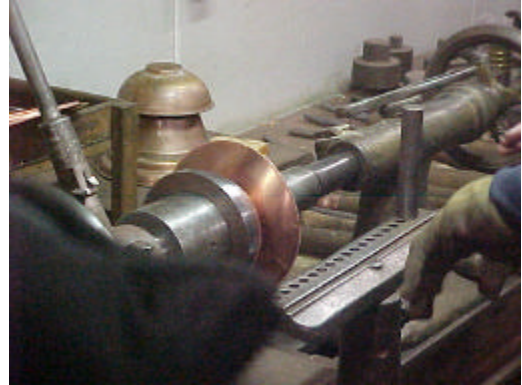
Copper sheet on lathe.
