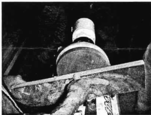
Rim sanded flat with sanding board.
