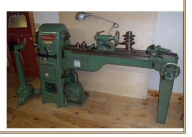
This is a 1970's vintage Rockwell Heavy Duty Variable speed lathe featuring 36" between centers with a 12" swing.
