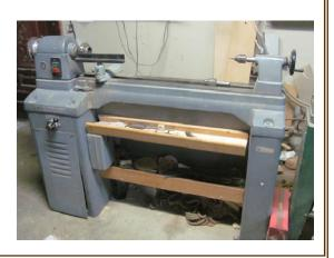
Model 46-111 with metal stand 1/3 hp motor 36" between centers and a 10" swing Good condition, except for a broken banjo
