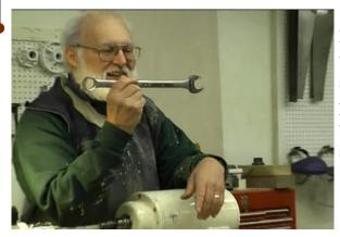
His discussion for the evening started with showing the tool he uses to make repetitive tenons it's an open end wrench with one side ground to parting tool edge. Place it on the tool rest and push forward until the ground edge engages then pull the handle up and move forward. In very short order you have a properly sized tenon. Al has home made sizes from 1/4" to 1 3/4".
