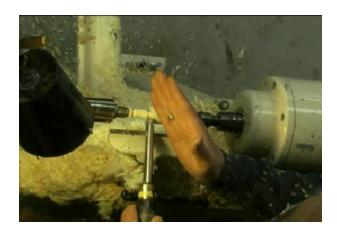
"if you cut like this" you see that the bevel is moving the point of attack to the left and a curve is developed.
